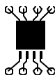
b) 105^\circ\text{C/W} when mounted on a .04\text{ in}^2 pad of 2 oz copper
